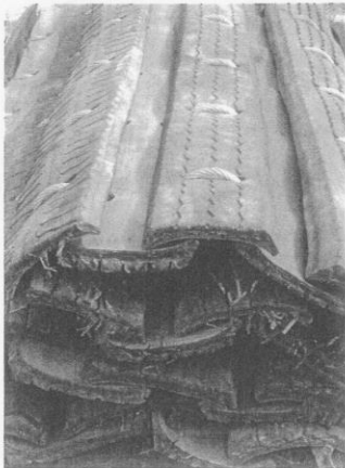
A typical blast mat weighs about 60 kilograms per square metre.
