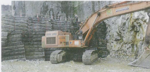
Blast mats are constructed from steel-belted treads of used car tyres, woven with steel cable.
